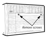
Remove one screw from each side of the case. Keep these ground/anti-theft screws so they may be replaced at the end of the installation.
